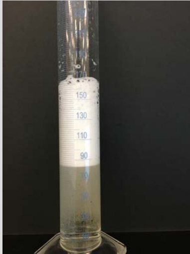
A commonly used dibasic acid product 1 minute after agitation in deionized water
