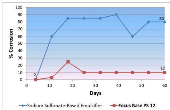
Figure 3: Corrosion (cast iron chip) of Emulsion Systems
